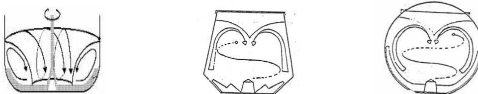
**Fig E: High-shear mixer-granulators with different mixing chamber design [4]**
