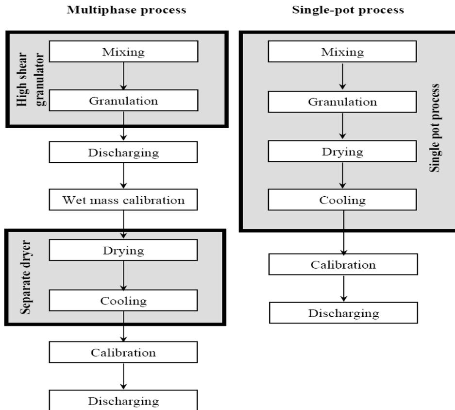
**Fig I: Granulating process: multiphase process vs single pot process**
