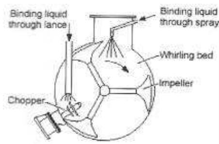
**Fig H2 horizontal shaft [6]**
