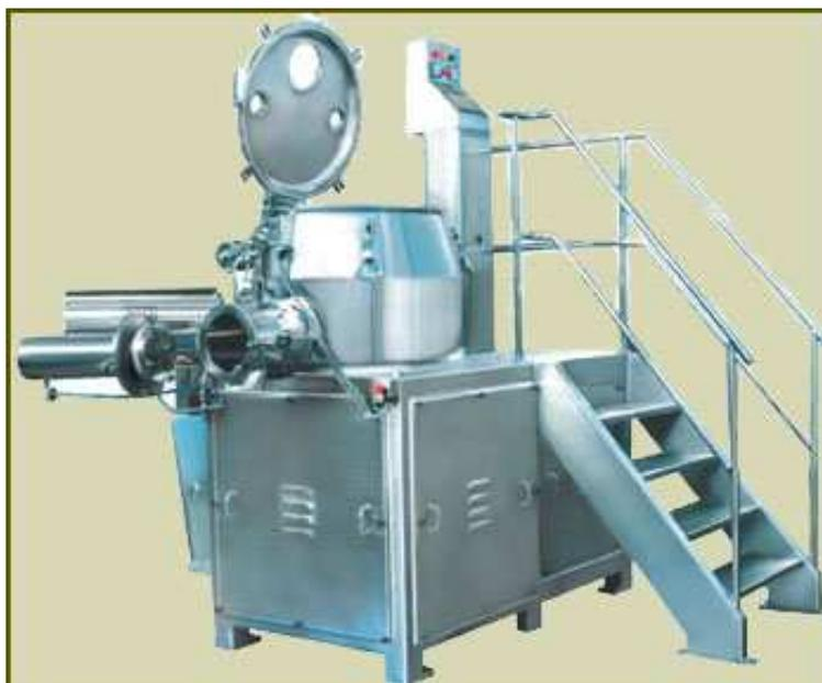
Fig.C: Rapid mixer granulator
