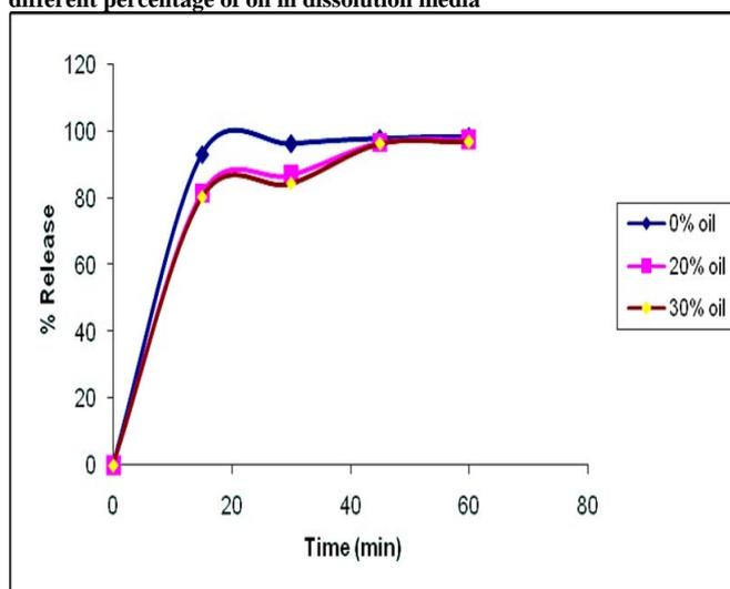
Fig. 3: Comparative dissolution profile of paracetamol at 75 rpm using different percentage of oil in dissolution media
